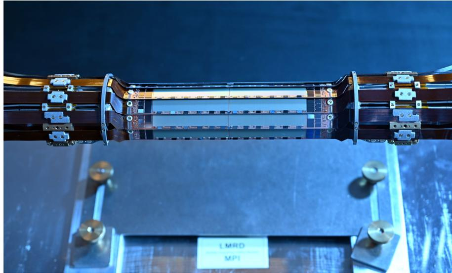
Since summer 2022 data taking, SuperKEKB and Belle II are in LS1, until fall 2023. Several improvements for accelerator complex, to reduce background and improve luminosity, and detector upgrades, such as installation of the complete two-layer vertex pixel detector. Details on SuperKEKB upgrade can be found [here](#)
