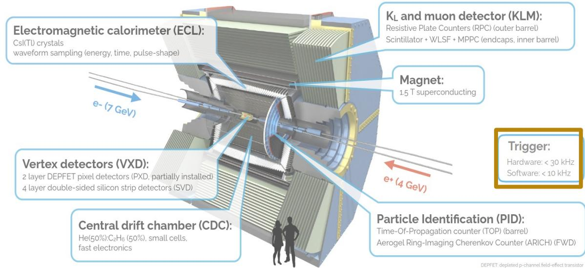
DEPFET: depleted p-channel field-effect transistor
