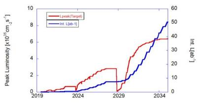
Projection of integrated luminosity delivered by SuperKEKB to Belle II
