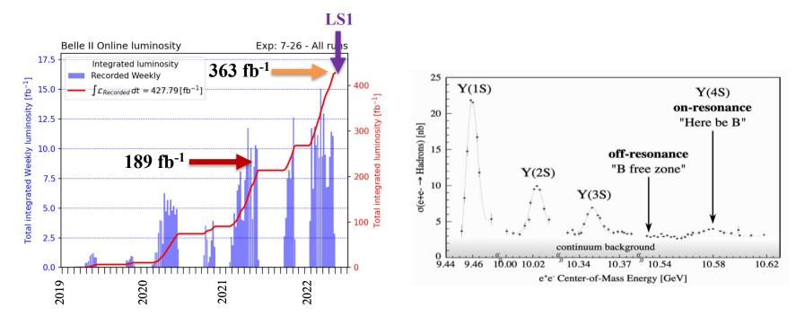
• **Currently:** Long Shutdown 1 (15 mos.) for detector upgrades and beam-pipe improvement
