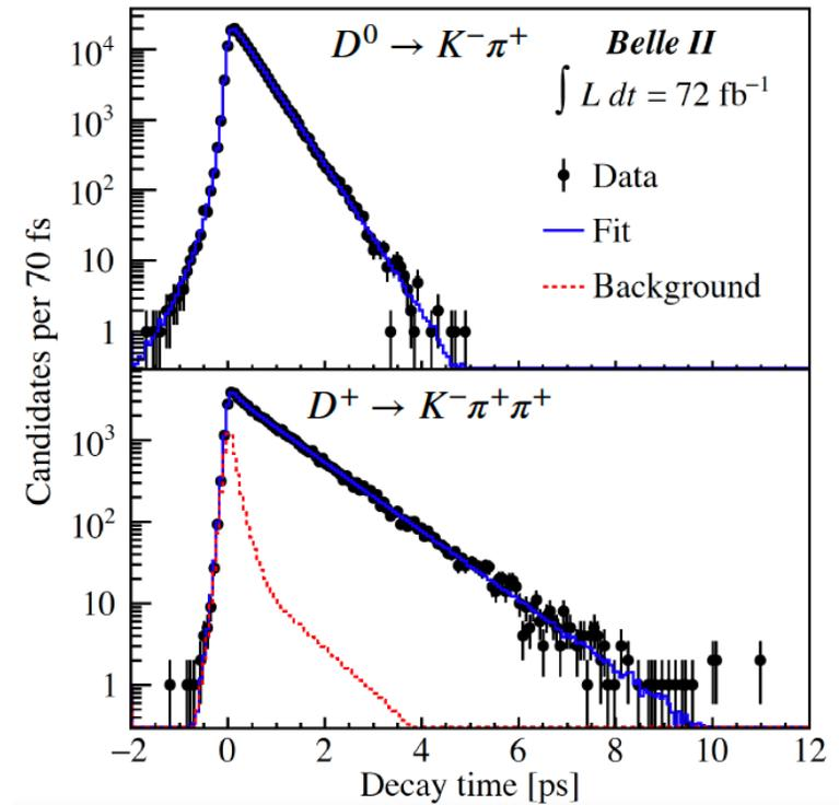
0.5% precision (incl. syst.) demonstrates excellent performance and understanding of Belle II vertex detector
