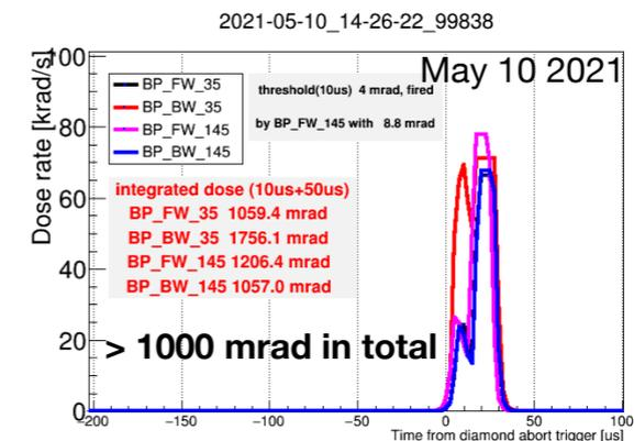
A significant beam loss at high beam current operation resulted in severe damage on a collimator or the vertex detector. Our abort system is not fast enough to protect such a sudden beam loss. → **A limitation toward higher beam current**
