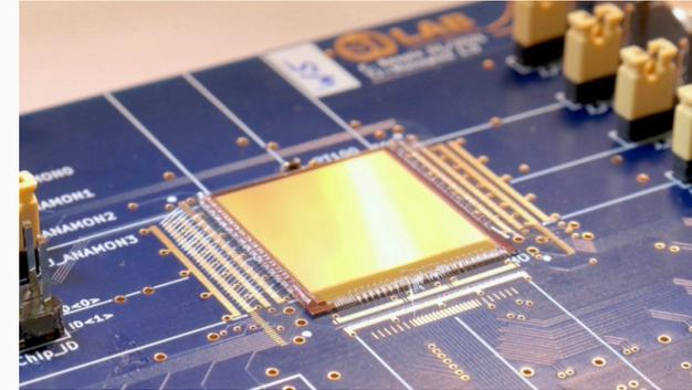
TJ-Monopix2: Proof-of-principle prototype of Belle II VTX
