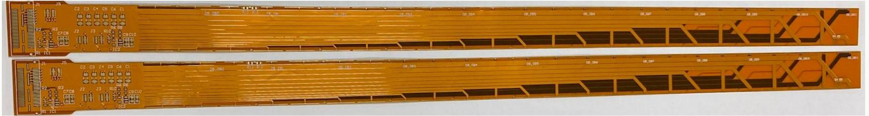
**First prototype** of the low power and signal bus available
