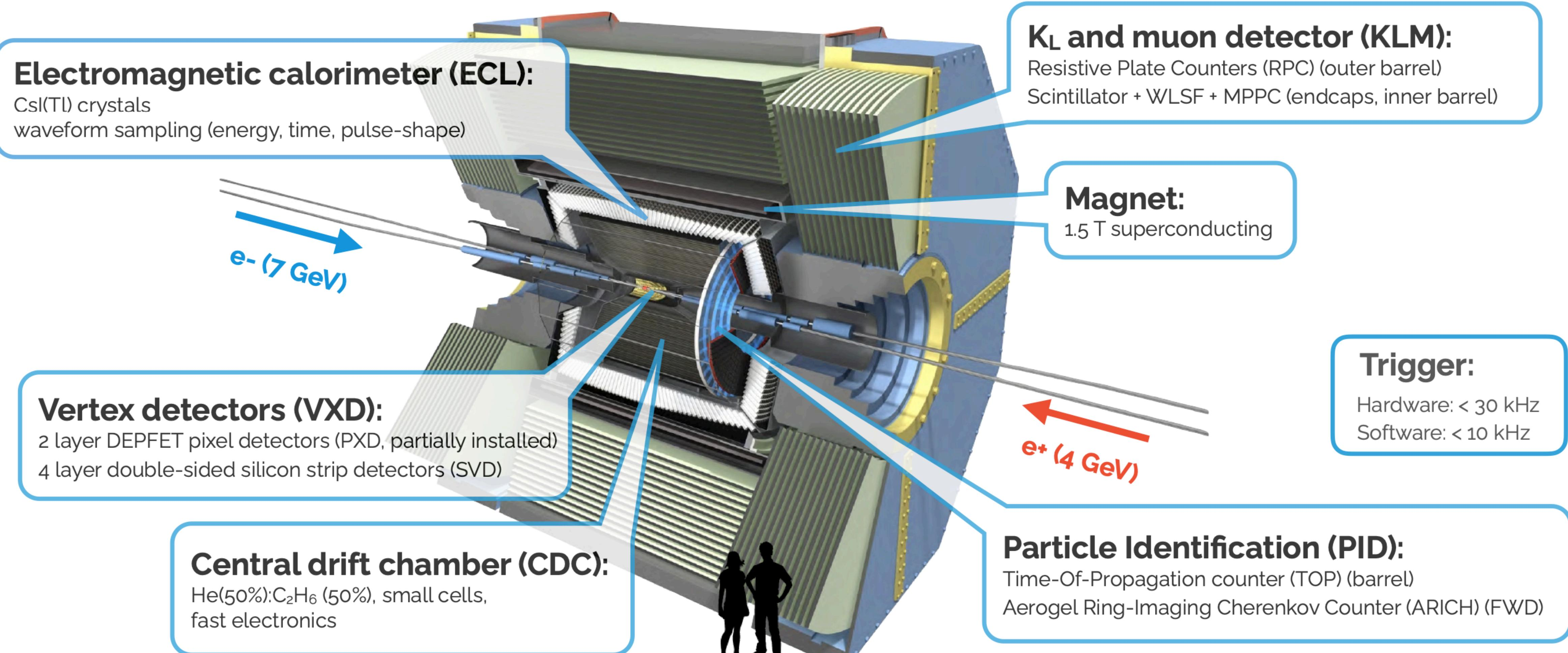
DEPFET: depleted p-channel field-effect transistor
