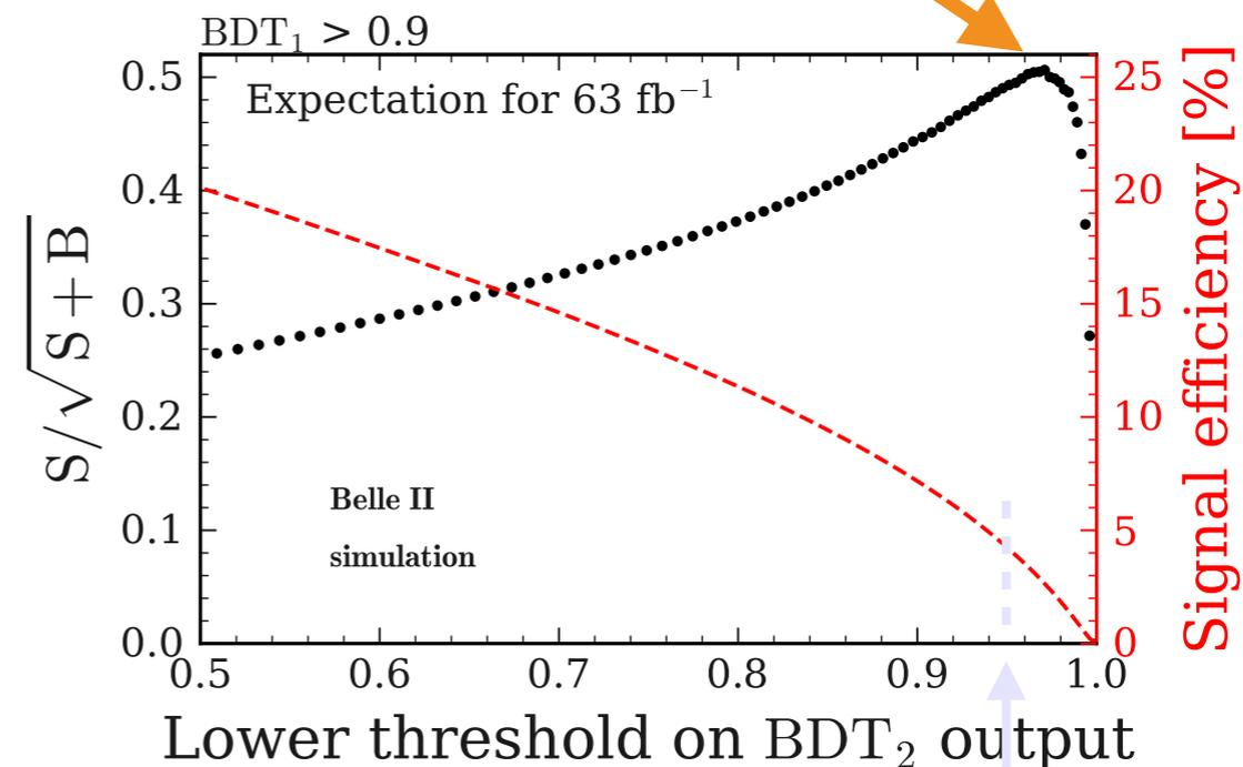
Signal Efficiency  $\sim 4.3\%$  (SM signal)
