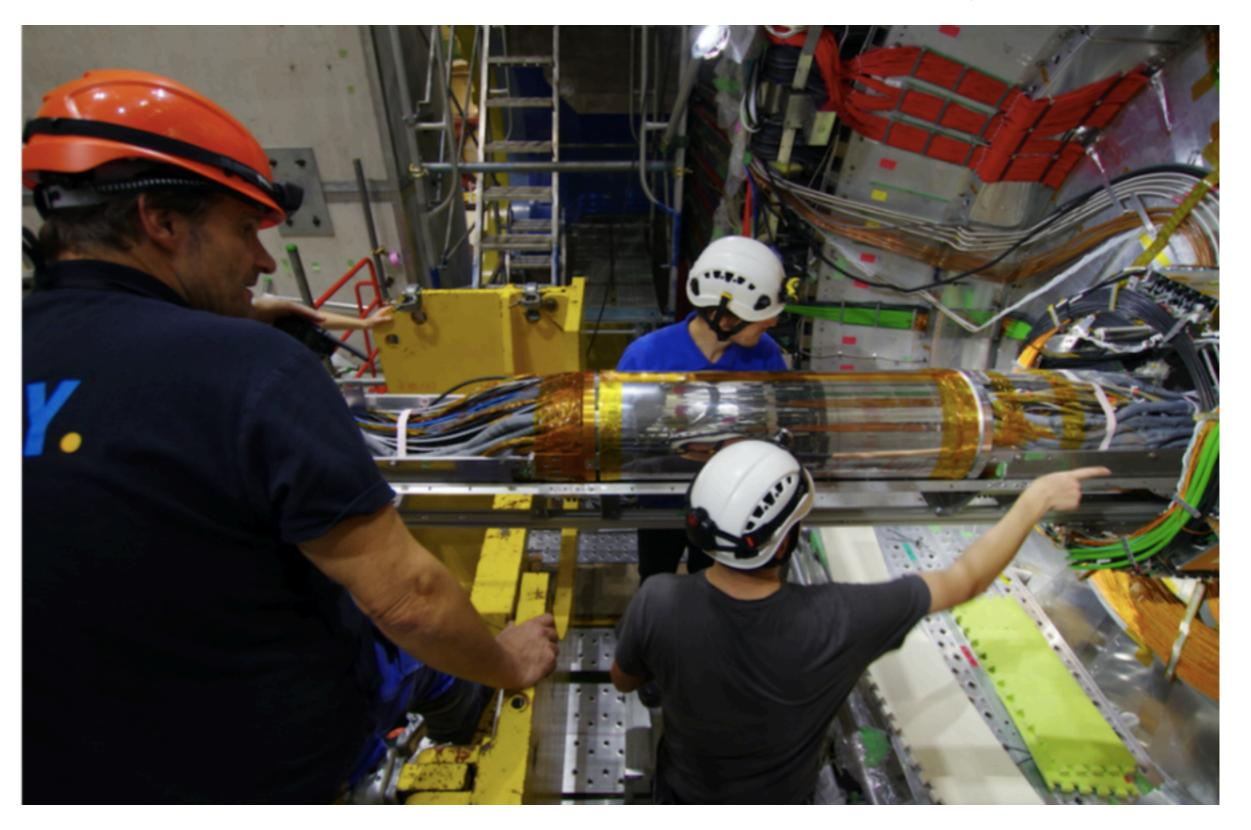
Pixel Detector (PXD): Layer 1 and partial Layer 2 Silicon-strip Vertex Detector (SVD): all 4 layers
