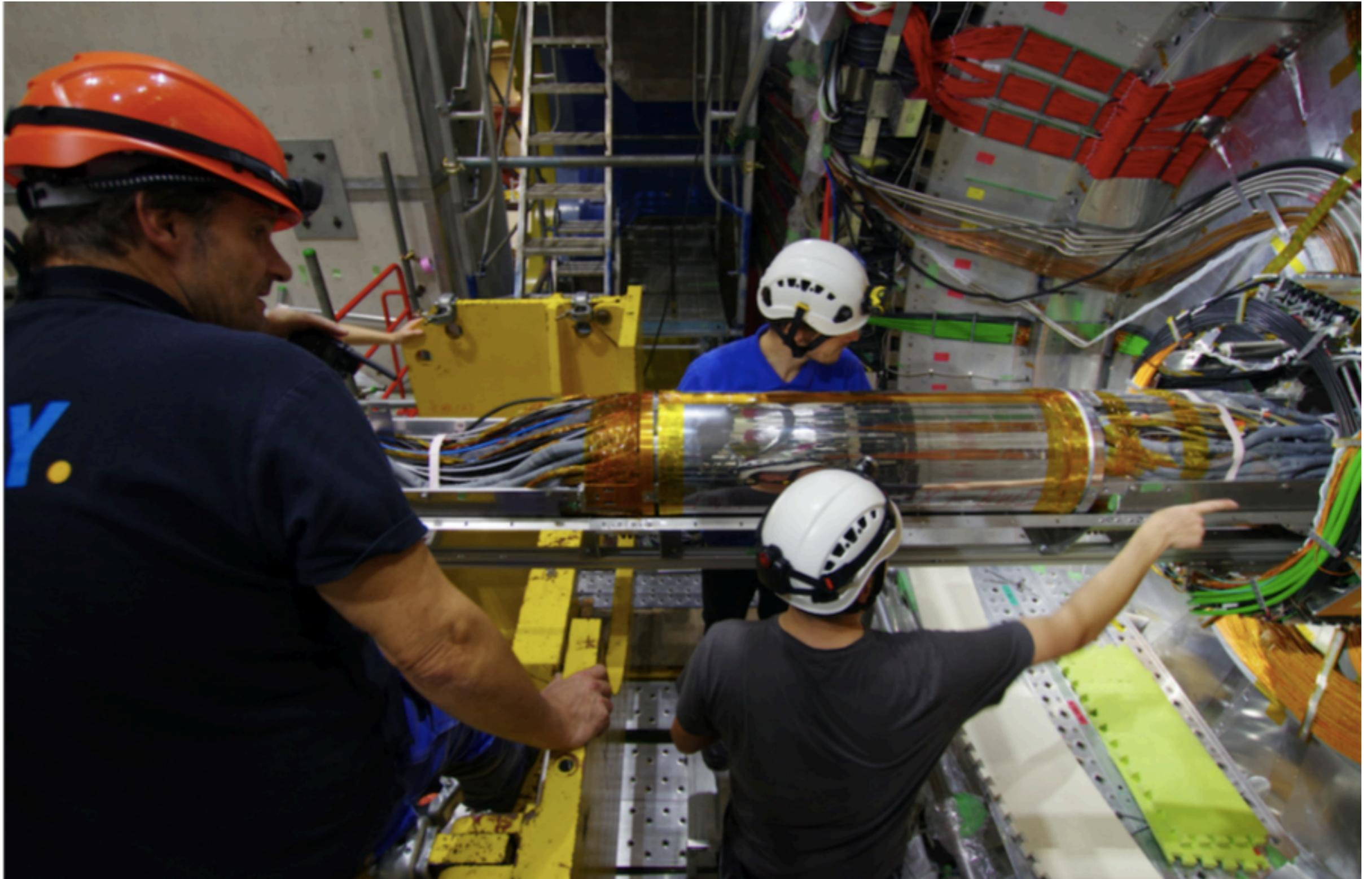
Pixel Detector (PXD): Layer 1 and partial Layer 2
