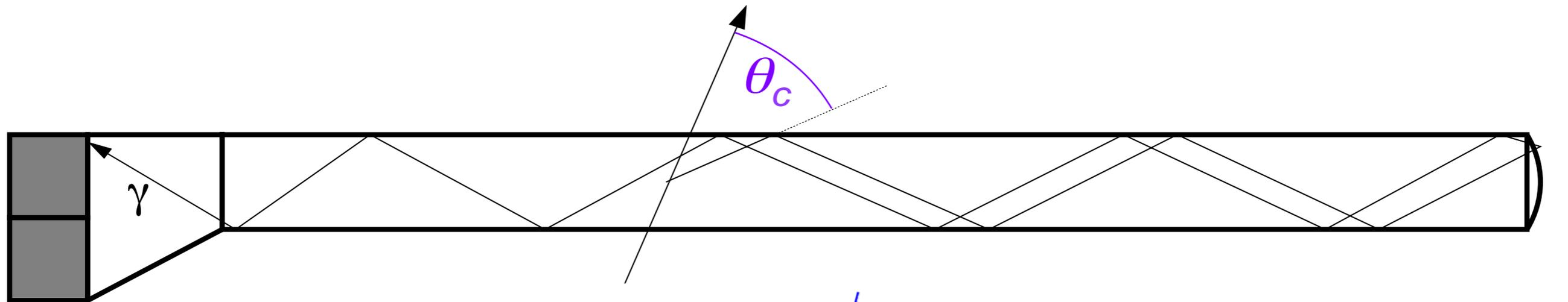
Čerenkov photons from **kaon** vs **pion** arrive at photosensors at different location and time
