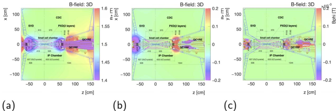
**Figure:** Magnetic field strength in x-z plane from simulation (model 1A): (a)  $B_z$  (b)  $B_r$  (c)  $B_\phi$  components. The Belle II detector drawing is overlaid.
