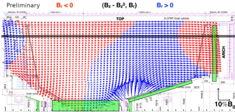
**Figure:** Initial estimate of field, created by accelerator development group, using Opera-3D (TOSCA). Green color highlights regions accessible when full magnetic system is present, black bar represents radial limit of whole volume measurement.
