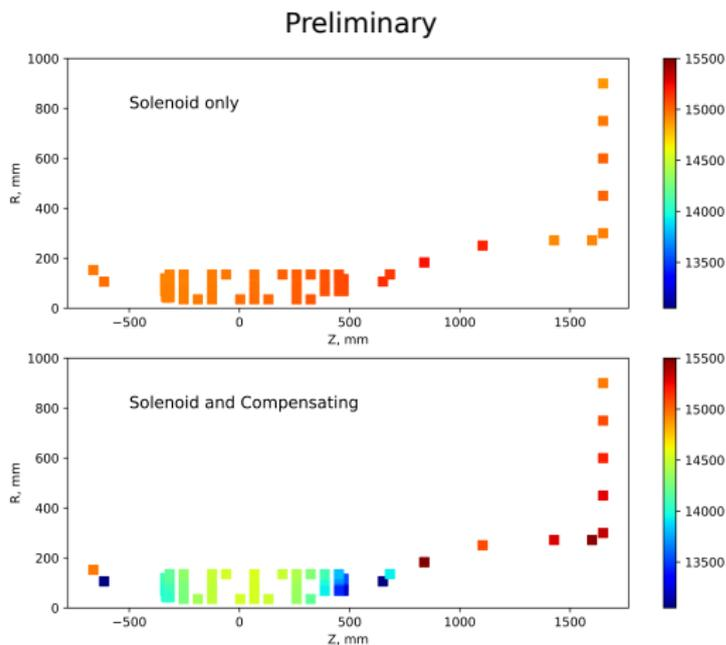
**Figure:** The B field generated by Belle II solenoid only and with compensating solenoids
