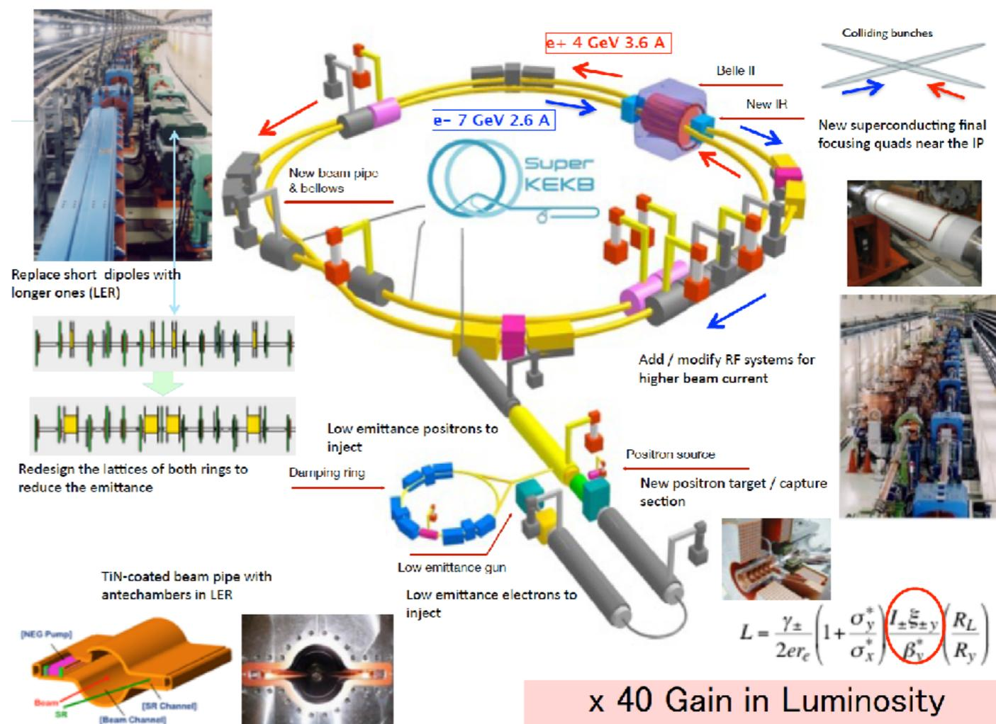
$$L = \frac{\gamma_{\pm}}{2e r_e} \left( 1 + \frac{\sigma_y^*}{\sigma_x^*} \right) \left( \frac{I_{\pm} \xi_{\pm y}}{\beta_y} \right) \left( \frac{R_L}{R_y} \right)$$
