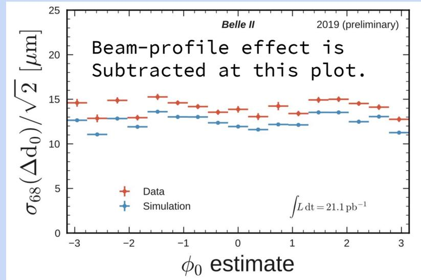
Impact parameter distributions in two-track events. Alignment and calibration are working well.
