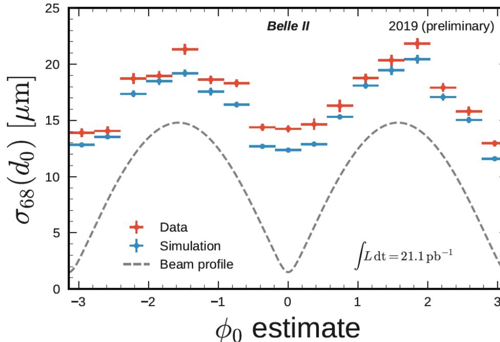
VXD resolution in impact parameter  $\sim 14 \mu\text{m}$
