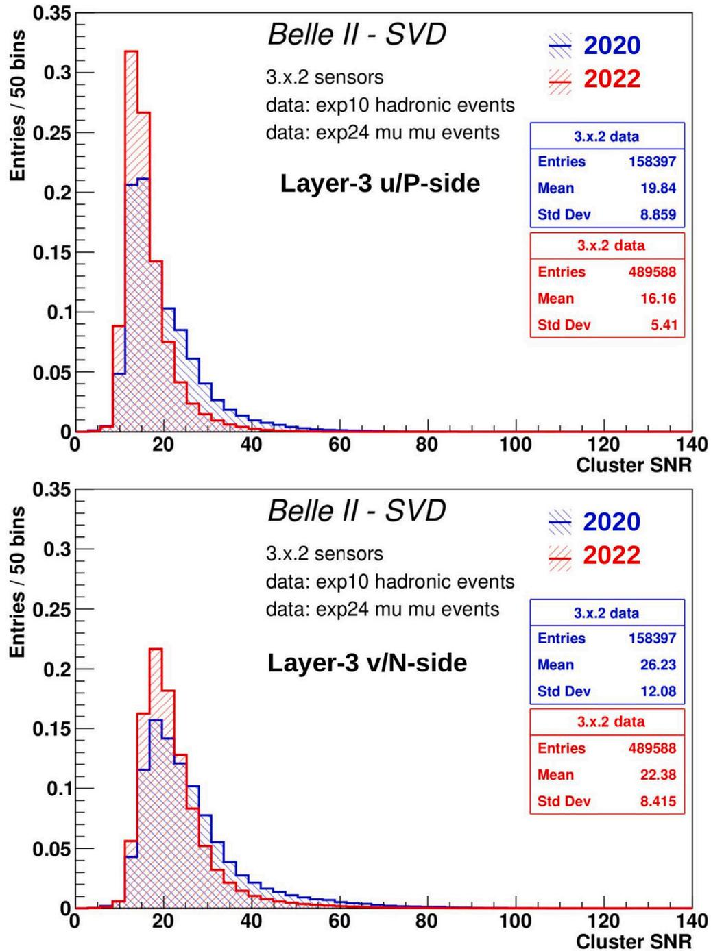
Fig. 2. Cluster SNR distribution for layer 3 u/P side (top) v/N side (bottom) for data collected in 2020 (exp10 data, in blue) and 2022 (exp24 data, in red). In the plots, the MPVs are approximately 15 (u/P side) and 18 (v/N side) for the 2020 data.
