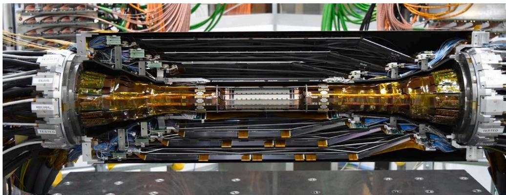
Fig. 3. Picture of the first SVD half-shell attached to PXD2.
