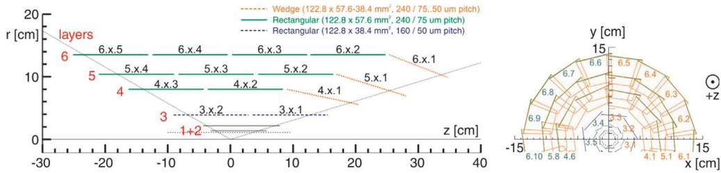
Fig. 1. Schematic view of the position of SVD layers and sensors.
