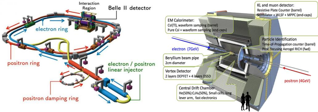
Figure 1: SuperKEKB accelerator (left) and Belle II detector (right).
