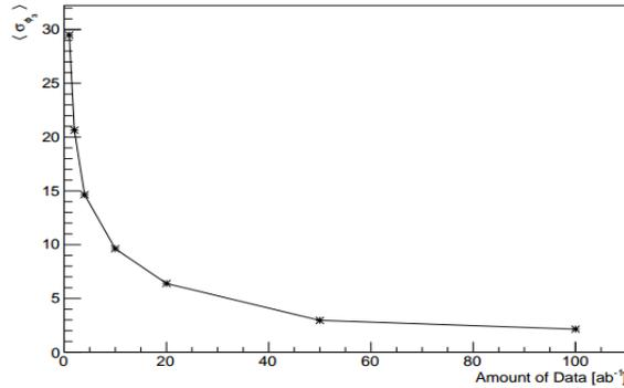
Fig. 2: Distribution between the expected  $\phi_3$  from  $B^+ \rightarrow D(K_S^0 \pi^+ \pi^-) K^+$  uncertainty versus luminosity accumulated by Belle II [9].
