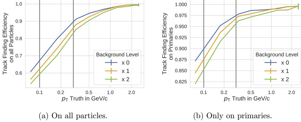
Figure 13: Track finding efficiency calculated for simulated  $\Upsilon(4S)$  events with different levels of beam-induced background relative to the expected level. Figure 13a is calculated on all trackable simulated particles, whereas Figure 13b only takes into account trackable particles from the primary interaction. The gray vertical lines indicate the typical transverse momentum of particles only trackable in the VXD (below left line) and with high efficiency in the CDC (above right line).
