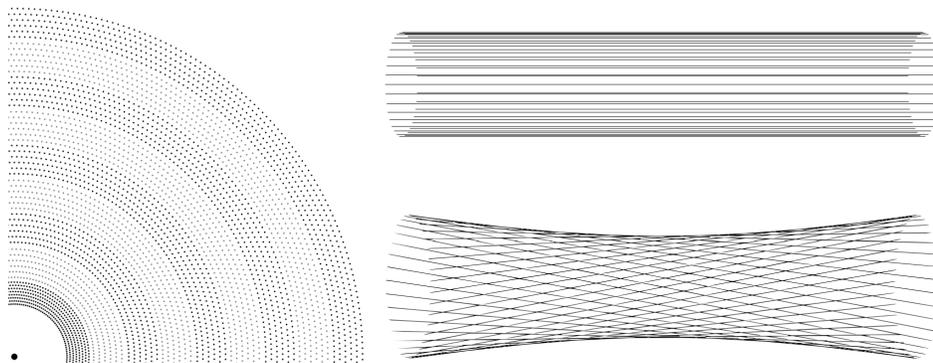
Figure 2: Left: A quadrant of a slice of the  $r$ - $\phi$  projection of the drift chamber. The innermost superlayer contains eight layers, all others contain six. Right: A visualization of stereo wires (bottom) relative to axial wires (top). The skew is exaggerated.
