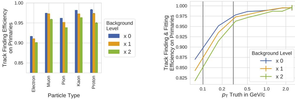
Figure 14: Finding efficiency by particle type and combined finding and fitting efficiency.
