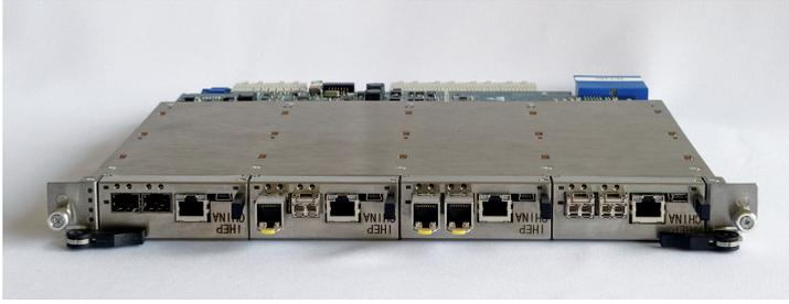
Figure 4.4: Photograph of the CNCB with 4 xFP cards installed. The plate on top ensure air flow when installed in the ATCA shelf.
