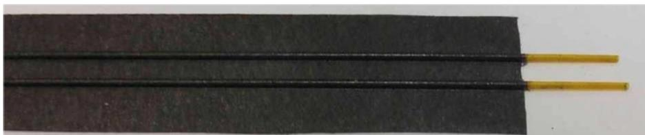
Figure 4.5: A prototype of the cold-plate for cooling. One coolant tube(golden) is connected to the cold plate(black) and turns 180° on the other end (not shown) so that the coolant flows in both directions and thus leaves on the same side it starts.
