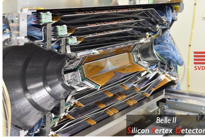
Figure 2.4: Belle II SVD with its complete set of four layers.
