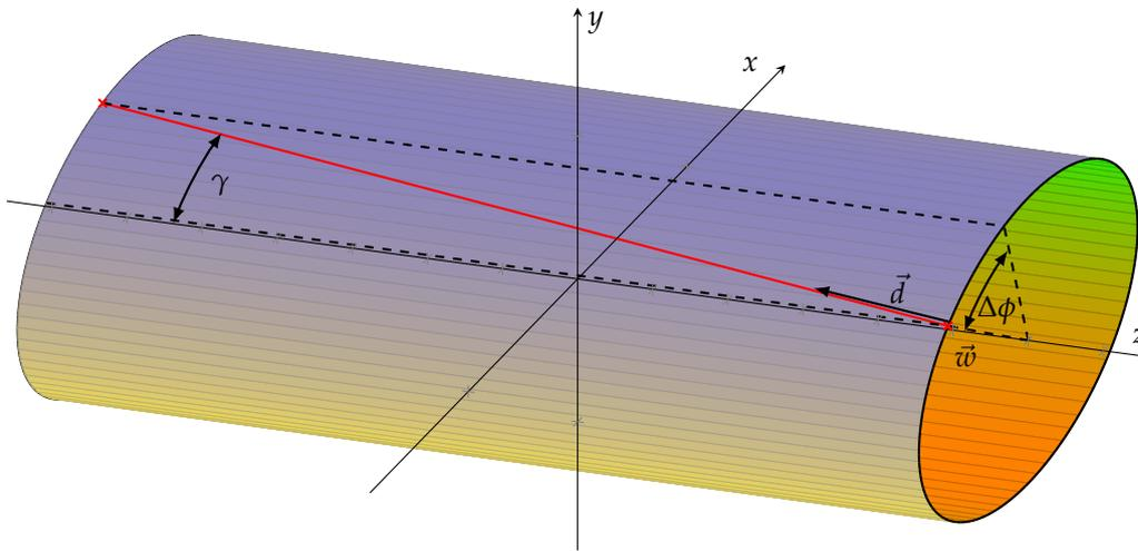
Figure 5.6.: Parametrization of a stereo wire as a straight line with a reference position  $\vec{w}$  and a direction vector  $\vec{d}$ . A stereo angle  $\gamma$  and the direction vector  $\vec{d}$  can be calculated from the  $\phi$ -shift  $\Delta\phi$  of the wire mounting positions at the forward and at the backward endplate.
