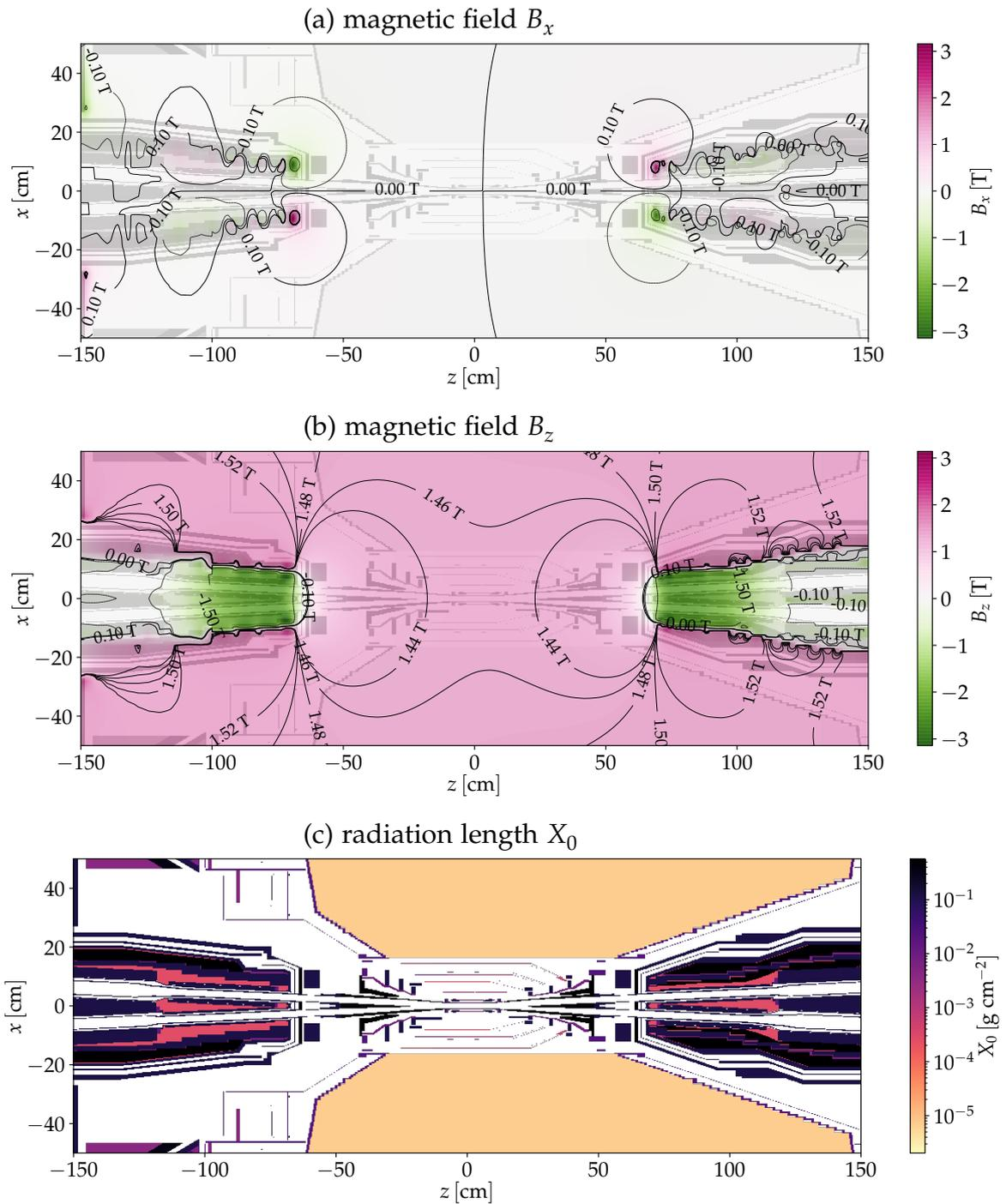
Figure 3.6.: (a) and (b) show a simulation of the Belle II 3D magnetic field in  $x$ -direction and in  $z$ -direction illustrating the distortions from the uniform 1.5T solenoid field in  $z$ -direction. (c) shows the simulated radiation length of the material budget. The magnetic field and radiation length correspond to a cut through the Belle II detector in the  $xz$ -plane.
