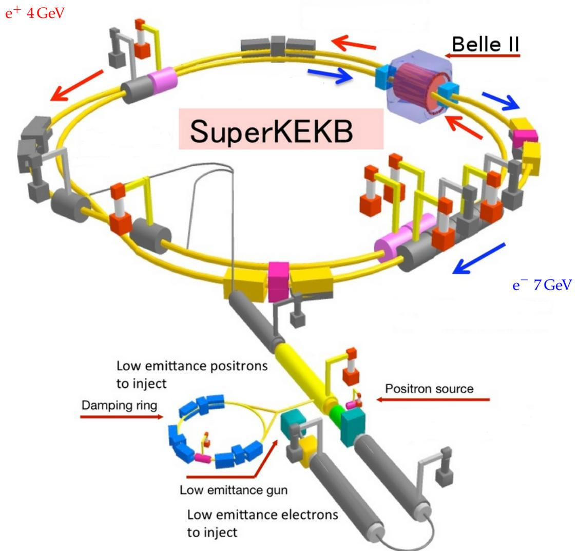
Figure 3.2.: Main structure of the SuperKEKB machine [42]. The  $e^-$  and  $e^+$  particles are injected into two separate rings and brought to collision in the interaction region, which is surrounded by the Belle II detector.
