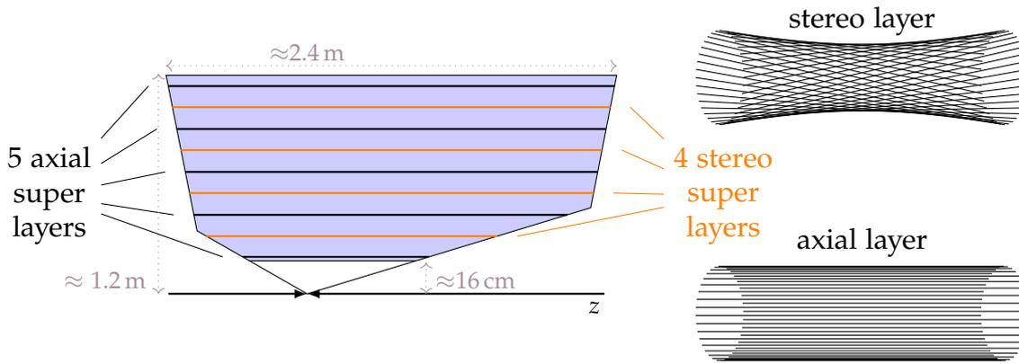
Figure 3.8.: Illustration of the alternating SL configuration in the CDC. Five axial SL are inclined with four stereo SL with a twist w.r.t. the  $z$ -axis.
