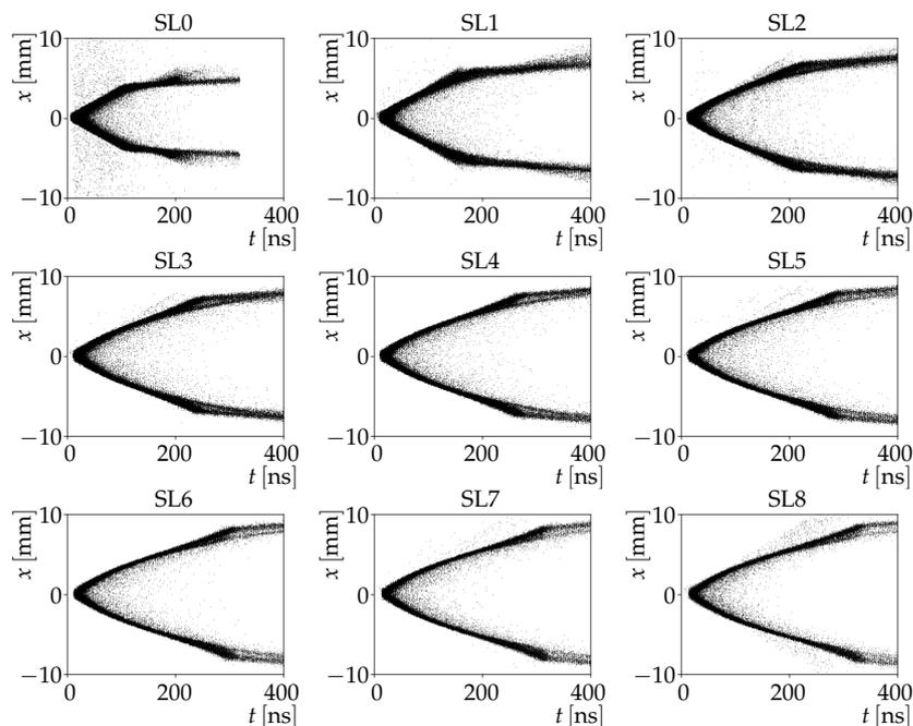
Figure 3.9.: Simulated  $xt$ -relation in the nine CDC SLs. The approximately linear regime is proportional to the cell sizes. The times are calculated from the simulated TDC counts after subtracting the  $t_{\text{wire}}^0$  of the wires.
