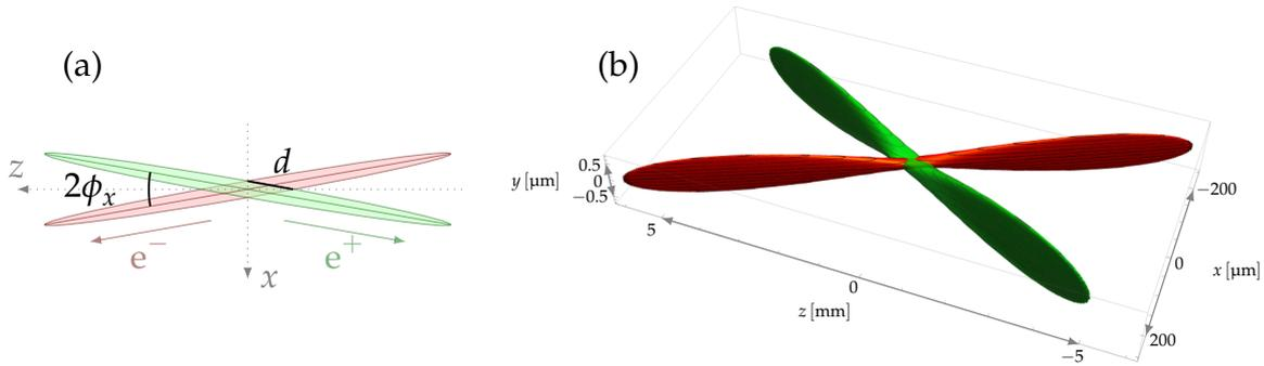
Figure 3.4.: (a) Bunch crossing at the Interaction Point (IP) of Belle II with the nano beam scheme in the  $xz$ -plane with the crossing angle  $2\phi_x = 83$  mrad and the effective bunch length  $d \approx 0.2$  mm. (b) Perspective view of the 3D bunch shape at the bunch crossing [52].
