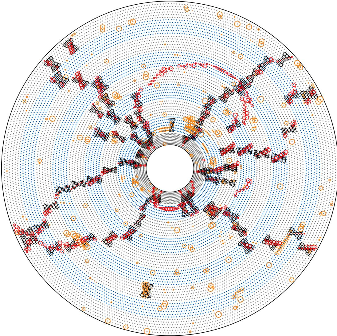
Figure 3.14.: Example event display of an  $Y(4S)$  event as seen after the TSF of the L1 CDC trigger [66]. CDC wires in axial layers are shown in gray, wires in stereo layers in blue. The CDC hits from the  $Y(4S)$  event are shown as red circles, background hits as orange circles. The found TSF are shown in black.
