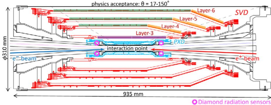
Figure 3: Schematic of the Belle-II vertex detector (VXD), the PXD layer is blue, and the four outer layers with red marks are the Silicon Vertex Detector (SVD).[2]
