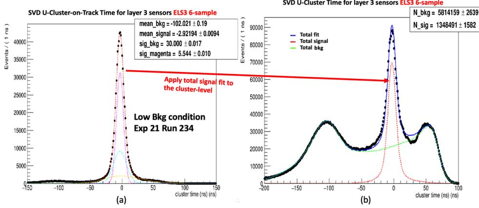
Figure 11: The total Gaussian fit to the 6-sample using ELS3 algorithm in the cluster-time plot.
