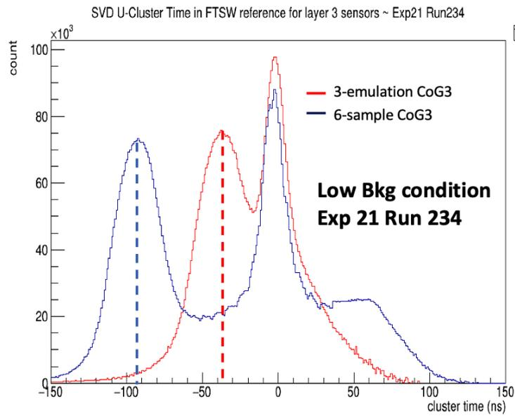
Figure 8: 3-sample emulation vs. 6-sample using CoG3 algorithm. Red curve is the CoG3 with 3-sample emulation mode; Blue curve is the CoG3 with 6-sample mode
