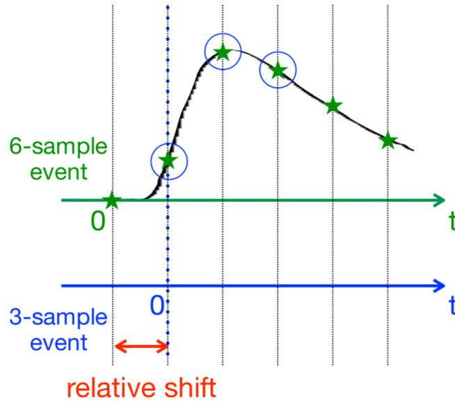
Figure 7: 3-sample emulation from 6-sample DAQ. Green stars are the 6-sample. Green stars with blue circles are the 3-sample chosen from the 6-sample with a relative shift[6]
