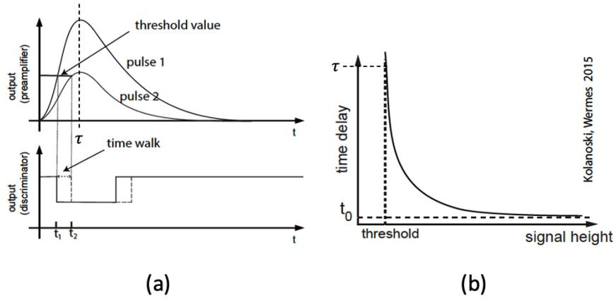
Figure 20: The procedure to get time delay plot. (a) upper plot is the analogue output and the lower plot is the digital output. (b) The time delay plot with varying signal height [9]
