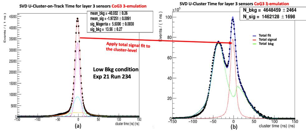
Figure 12: The total Gaussian fit to the 3-sample emulation using CoG3 algorithm in the cluster-time plot
