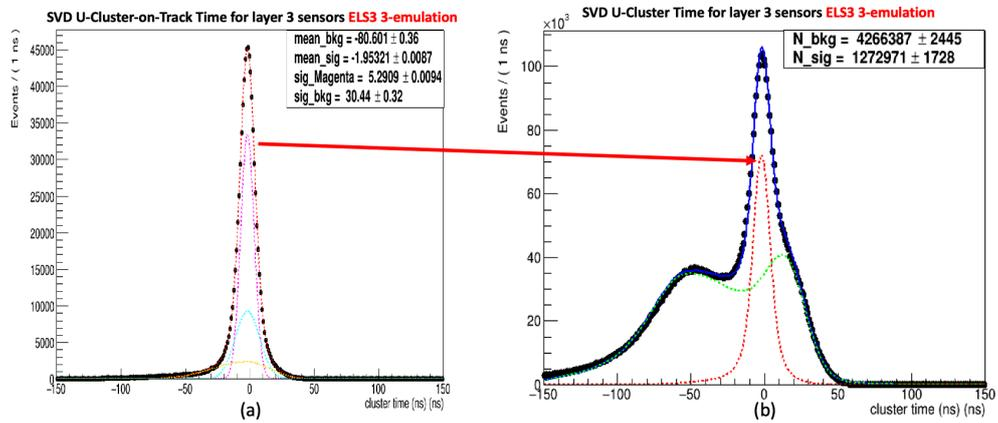
Figure 13: The total Gaussian fit to the 3-sample emulation using ELS3 in the cluster-time plot
