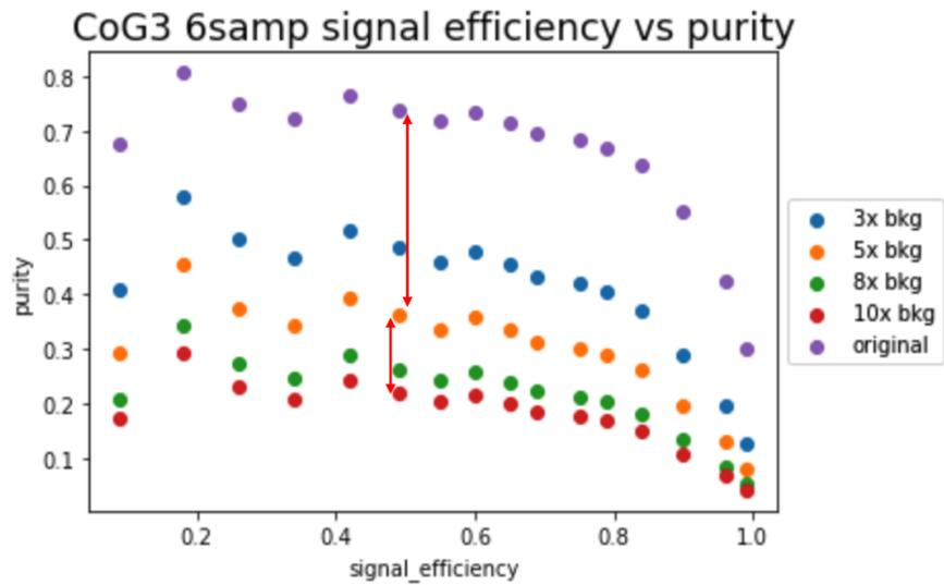
Figure 17: Purity vs. signal efficiency plot for 6-sample using CoG3 with increasing background events.
