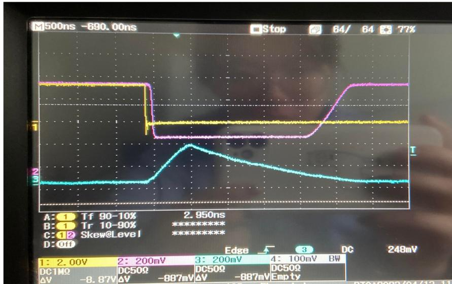
Figure 23: The output of the analogue, digital and injected pulse from MIMOSIS-Fast shown on the oscilloscope. yellow line: injected pulse; magenta line: digital output; blue line: analogue output. The width of each grid on the screen is 500ns.
