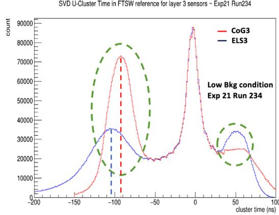
Figure 6: The 6-sample DAQ: CoG3 vs. ELS3 tested on low background condition data collected in 2021. The red line is the 6-sample readout mode using GoG3 algorithm for cluster time reconstruction, the blue line using ELS3 algorithm. The two green circles represent the beam-induced background peaked at the positive and negative sides.
