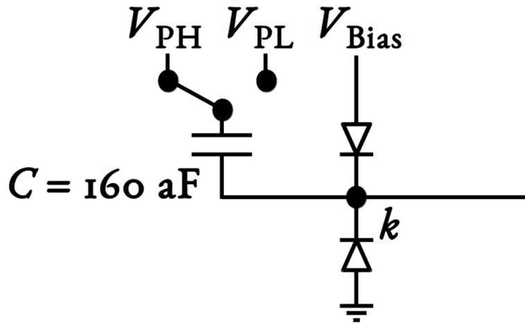
Figure 21: Schematic sketch of the charge injection system in MIMOSIS-Fast
