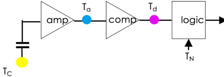
Figure 19: The signal propagation in each pixel in a CMOS sensor:  $T_c$  is the collision time;  $T_a$  is the analogue pulse passes the detection threshold;  $T_d$  is the digital pixel output switch from 0 to 1;  $T_d$  is the time when frame N starts )
