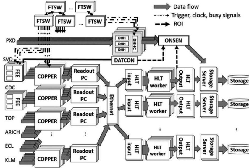
Figure 4: Data Acquisition System for the Belle II[4]
