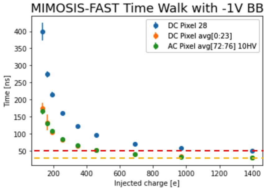
Figure 24: The time delay plot for the MIMOSIS-Fast
