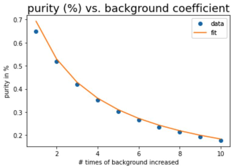
Figure 18: The purity vs different times (1 to 10 times)increased selected background at 80% signal efficiency. The orange curve is the  $constant/(constant + x)$  fit to the blue dots where constant equals to 2.25.
