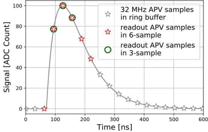
Figure 5: Example of sampling in “multi-peak” mode of the APV25. The gray curve is the signal waveform. The grey stars represent the sampled signal stored in the ring buffer using 32 MHz sampling clock. The red stars are the 6 consecutive samples read out, and the red stars with green circle are the 3 consecutive samples chosen from the 6-sample mode with a relative shift[2]
