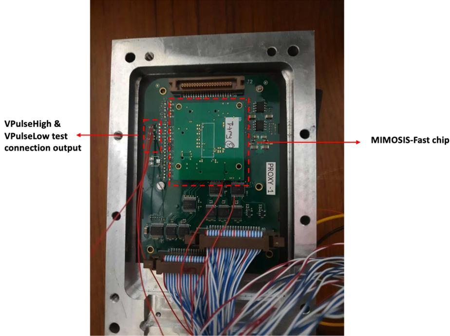
Figure 22: The set-up of the proximity board in the MIMOSIS-Fast study. The proximity board has different connections for test outputs, VPulseHigh and VPulseLow outputs are marked in the plot. The MIMOSIS-Fast chip is located at the center of the proximity board.
