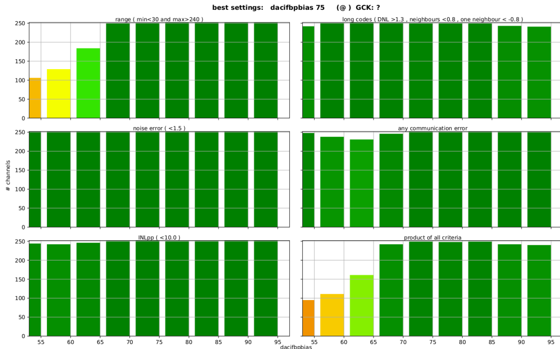
Figure 6.10: Parameter sweep over IFBPBias. For the five possible features the number of good channels is calculated and put into individual plots. The sixth plot shows the product of all criteria and an optimal setting is extracted, suggested and printed as the headline by the analysis script.
