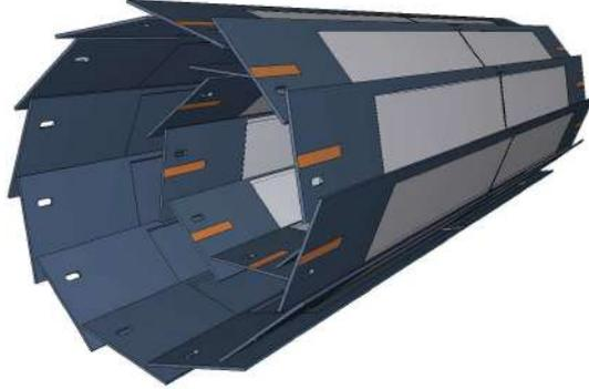
Figure 2.4: View of the two-layers DEPFET Pixel Detector.
