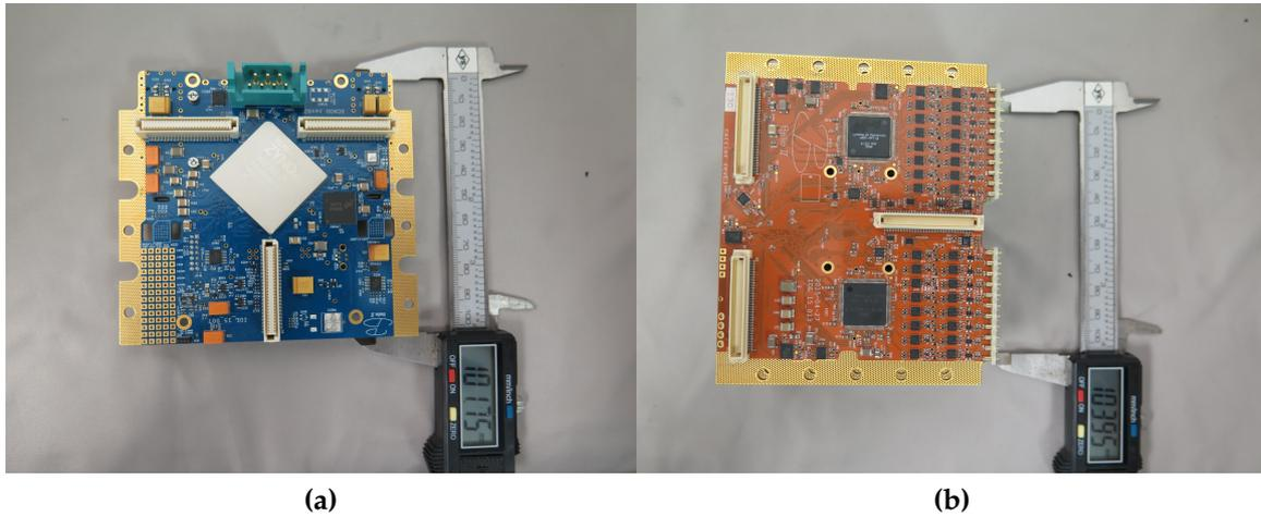
**Figure 2.14.:** SCROD with Xilinx Zynq FPGA, three mezzanine and one power connector shown (left); Carrier with two of four IRSX ASICs shown, as well as three mezzanine connectors and top edges of POGO pin assemblies to the right (right); One SCROD and four carriers constitute one electronic readout module ("boardstack")
