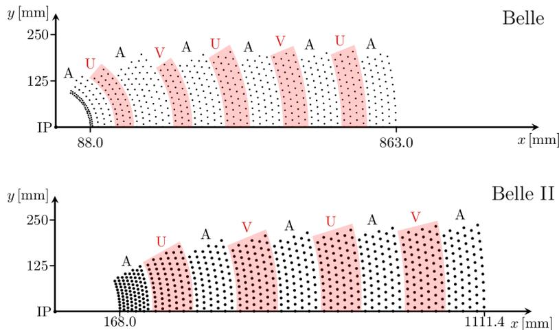
**Figure 3.8:** Layer configuration of the CDC at Belle (top) and at Belle II (bottom). The letter A stays for axial superlayers; the letter U for stereo superlayers with positive stereo angle; and the letter V for stereo superlayers with negative stereo angle.
