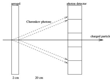
**Figure 3.13:** Proximity focusing ARICH - principle
