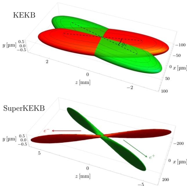
**Figure 3.3:** Schematic view of the beam crossing at KEKB (top) and at SuperKEKB (bottom). The crossing angle is shown in the top. The beam directions are shown in the bottom scheme. The size of the interaction region in  $z$ -direction at KEKB was around 10 mm, while at SuperKEKB it is around 0.5 mm
