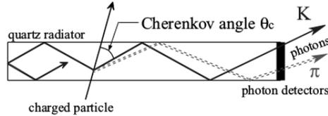
Figure 3.11: Schematic side-view of TOP counter and internal reflecting Cherenkov photons.
