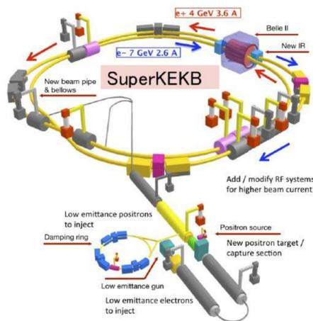
Figure 3.1: A schematic representation of the SuperKEKB asymmetric energy  $e^+e^-$  collider
