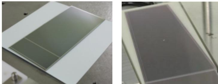
Figure 6.6: Rectangular (left) and trapezoidal (right) sensors.
