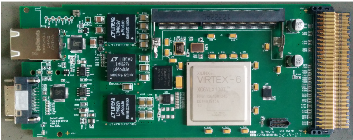
Figure 2.8.: DHE Version 3.2 with removed RAM. On the left side there are the Infiniband and RJ45 connectors to the PXD module and on the right side is the connector to the rag. [16]
