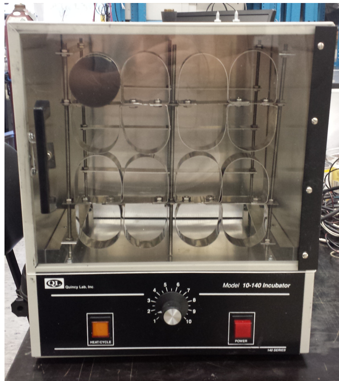
Figure B.12: Incubator used in experimental setup. Version shown has UVT window installed, and contains mechanical support structure for the aging measurements in chapter 7.
