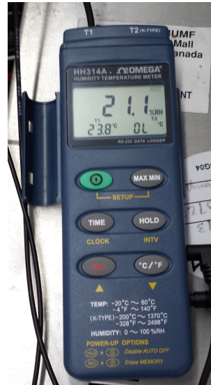
Figure B.11: Temperature and humidity reader base for measurements within the dark box.
