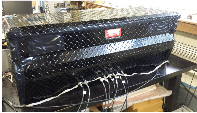
Figure B.10: The dark box, prepared by Chelsea Dunning, that was used for all but the most preliminary measurements.
