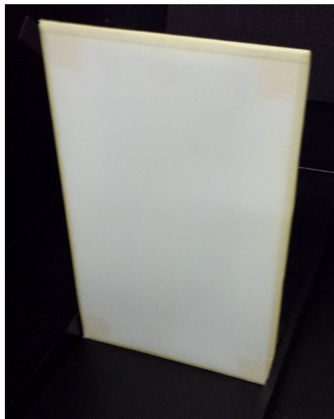
Figure B.8: Diffuse reflective screen used in excess noise measurements of chapter 6.
