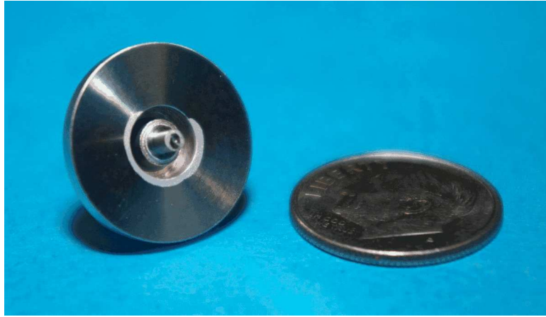
Figure 3.7: Test model of a pick-up electrode for the beam position monitor at the IP chamber.
