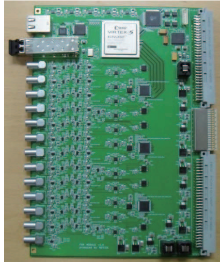
Figure 12.15: A photograph of 6U-VME type FAM prototype board
