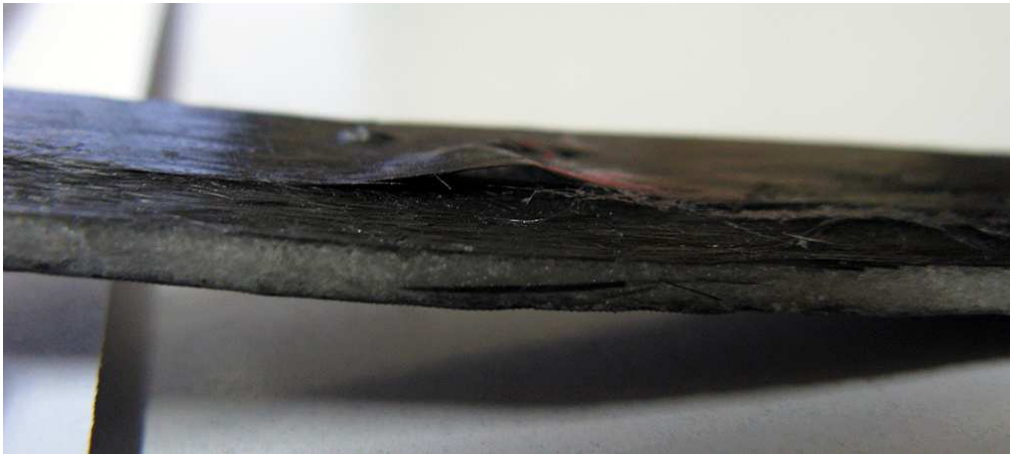
Figure 5.18: Delamination caused by applying excessive forces on both ends.
