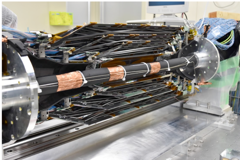
Completion of first SVD clam-shell (Jan 2018)
