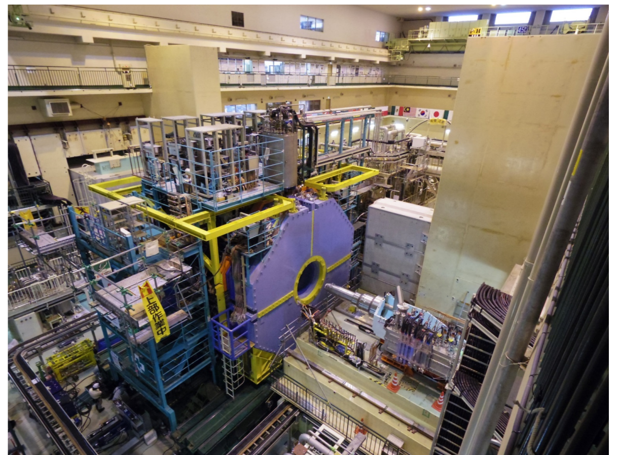
Belle II roll in: 1400 tons, 8m x 8m, moved 13m horizontally
