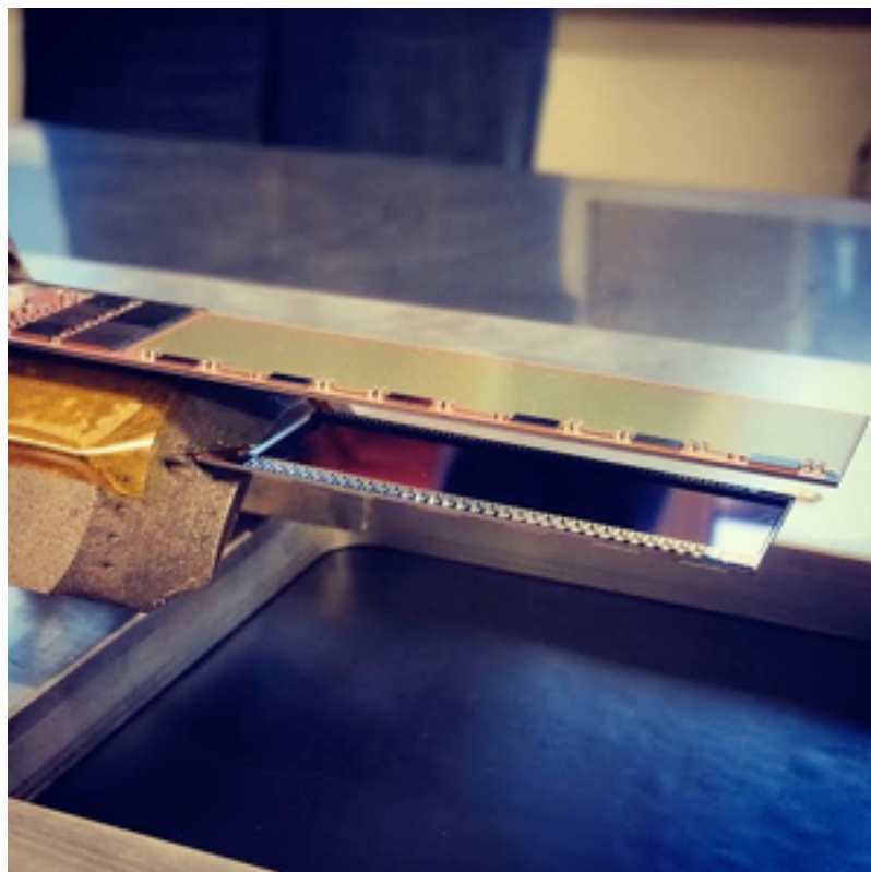
Test full-sized PXD modules in a beam.
