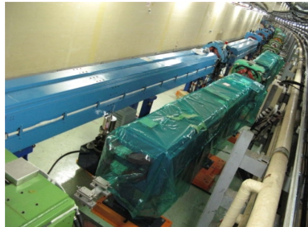
100 new LER bending magnets
