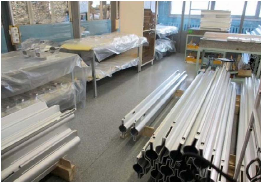
LER beam pipe with ante-chamber and Ti-N coating
