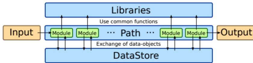
FIGURE 4.3: Schematic diagram of the general execution of modules chained into a path via a Python steering file. The modules operate event-by-event and use functionality provided by libraries and exchange data-objects via the common DataStore [13]
