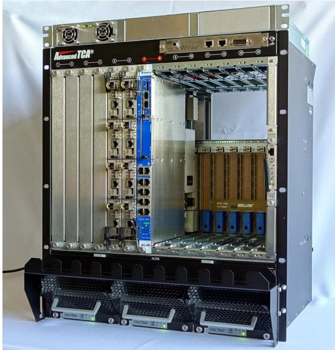
Figure 4.1: Photograph of a 14-slot, full-mesh ATCA shelf (Schroff 11592-402 [90]). ATCA carrier boards with four single, full-size AMC cards are present in slots 5 and 6. A base-channel GbE switch with two single, mid-size AMC cards is present in the first hub slot (slot 7). The right half of the shelf is left open to show the backplane with the blue power connector (Zone 1) and the fabric- and base-channel connector (Zone 2). The open space above the backplane can be used for the custom RTM connector (Zone 3). A 1 kW, 48 V power supply sits on top of the shelf. The Shelf Manager is plugged into a dedicated bay right of ATCA slot 14.
