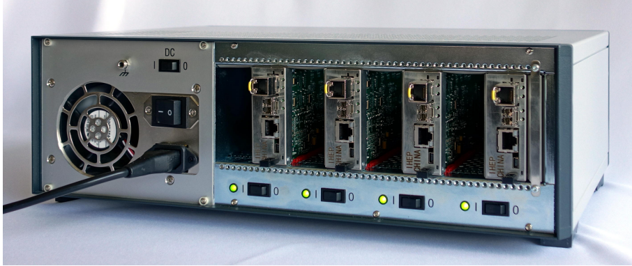
Figure 4.2: Photograph of a 4-slot MicroTCA shelf with fixed backplane connections between the AMC ports of the slots (Schroff 11850-013 [92]). A single, full-size AMC card is plugged into each slot. The slots in this shelf are extra-wide to allow access to the cards for testing purposes.
