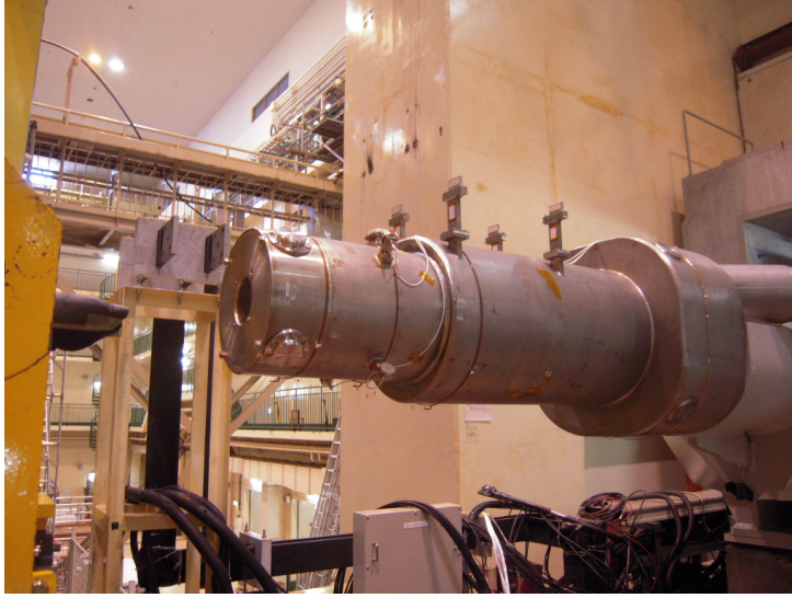
Figure 5.3: Cryostat for compensation solenoid and QCS
