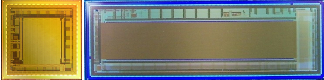
Figure 5.18: (Left) Picture of the DuTiP1 ( 6 \times 6 \text{mm}^2 ). (Right) Picture of the DuTiP2 ( 6 \times 17.2 \text{mm}^2 ).
