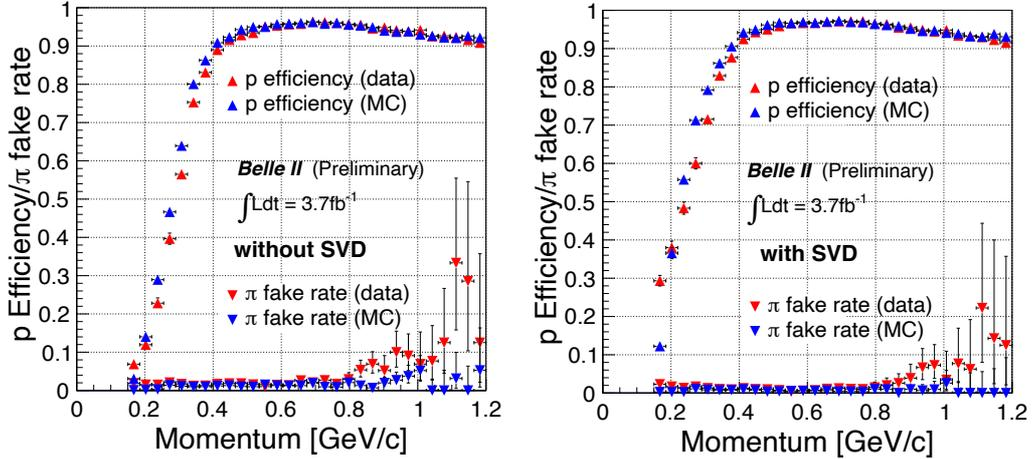
FIG. 7.  $p$  efficiency and  $\pi$  fake rate vs. momentum without (left) and with (right) SVD  $dE/dx$  information. To assess the impact of this information to the overall PID, we plot the efficiency and fake rate as a function of momentum applying a requirement on the PID likelihood  $\mathcal{L}(p/\pi) > 0.6$ . The study shows an improvement in proton efficiency after adding SVD  $dE/dx$  information.
