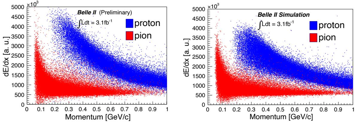
FIG. 4. Scatter plot of  $dE/dx$  of proton and pion as a function of their momentum in data (left) and MC (right) events from the  $\Lambda$  sample. The two-dimensional distributions of  $dE/dx$  vs. momentum show a clear separation between different particles in the low momentum region, and are uploaded to the calibration database.
