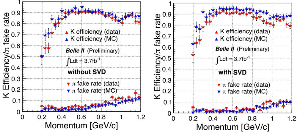
FIG. 6.  $K$  efficiency and  $\pi$  fake rate vs. momentum without (left) and with (right) SVD  $dE/dx$  information. To assess the impact of this information to the overall PID, we plot the efficiency and fake rate as a function of momentum applying a requirement on the PID likelihood  $\mathcal{L}(K/\pi) > 0.5$ . The study shows an improvement in kaon efficiency after adding SVD  $dE/dx$  information.
