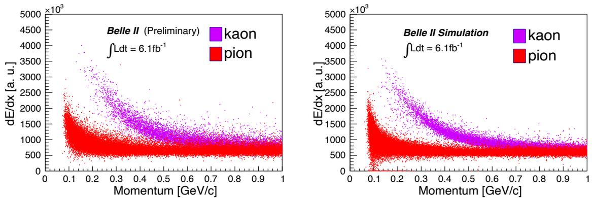
FIG. 3. Scatter plot of  $dE/dx$  values of charged pions and kaons as a function of their momentum for data (left) and MC (right) events from the  $D^*$  sample. The two-dimensional distributions of  $dE/dx$  vs. momentum show a clear separation between different particles in the low momentum region, and are uploaded to the calibration database.
