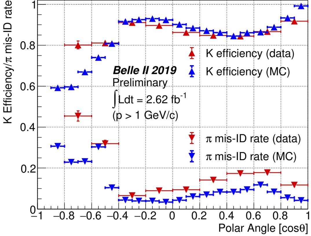
FIG. 7: Kaon efficiency and pion mis-ID rate for the PID criterion  $\mathcal{R}_{K/\pi} > 0.5$  using the decay  $D^{*+} \rightarrow D^0[K^-\pi^+]\pi^+$  in the bins of polar angle (laboratory frame) of the tracks which have laboratory frame momentum greater than  $1 \text{ GeV}/c$ . Note that the acceptance regions of CDC, TOP and ARICH in polar angle ( $\cos\theta$ ) are  $[-0.87, 0.96]$ ,  $[-0.48, 0.82]$ , and  $[0.87, 0.97]$ , respectively.
