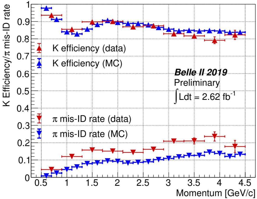
FIG. 4: Kaon efficiency and pion mis-ID rate for the PID criterion  $\mathcal{R}_{K/\pi} > 0.5$  using the decay  $D^{*+} \rightarrow D^0[K^-\pi^+]\pi^+$  in the bins of laboratory frame momentum of the tracks.
