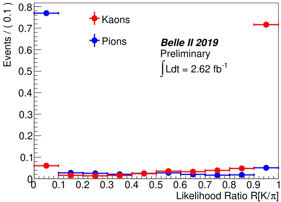
FIG. 1:  $\mathcal{R}_{K/\pi}$  distribution.  $K$  and  $\pi$  tracks are tagged from the charge of the slow  $\pi$  (daughter of  $D^{*+}$ ) in the decay  $D^{*+} \rightarrow D^0[K^-\pi^+]\pi^+$ .
